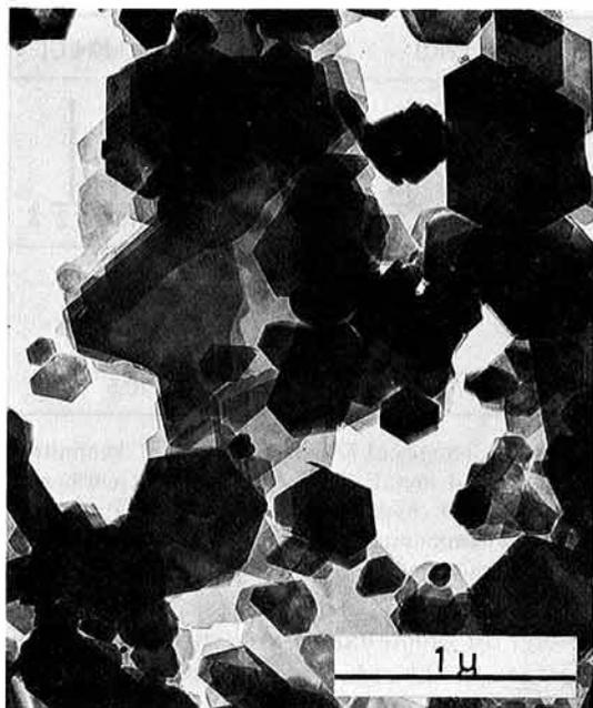
Plate 1. Electron micrograph of kaolinite from geological deposit
