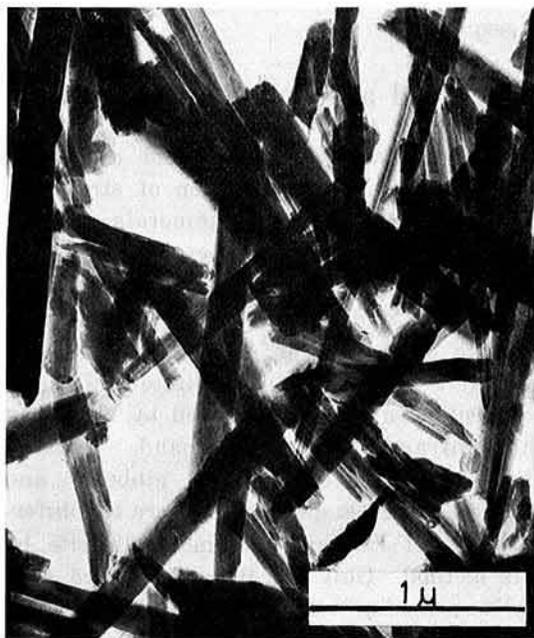
Plate 2. Electron micrograph of metahalloysite from geological deposit.
