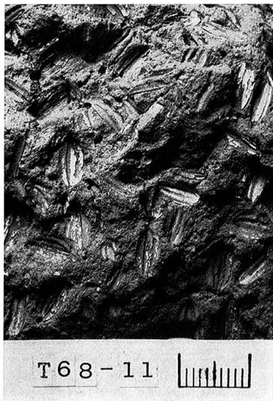
Fig. 1. Rice husks contained in a brick
