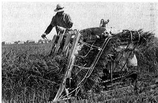
Fig. 1. Prototype high capacity combine, manufactured for trial in IAM —IAM HT-711—
