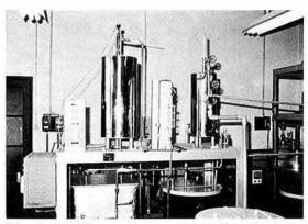
Fig. 3. Continuous flow system pilot plant for chemical isomerization
