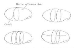
Fig. 1. Examples of cracked kernel graded as damaged kernel for official inspection in Japan.
