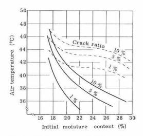
Fig. 2. Relation among initial moisture content, air temperature and crack ratio in thin layer drying
