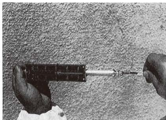
Fig. 1. Method of measuring physical strength of root.
