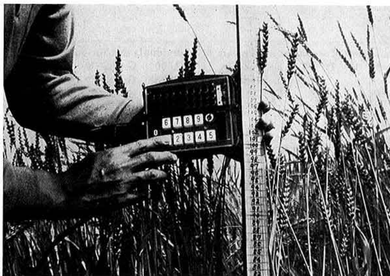
Fig. 3. Panel of operation board for data transmitting.
