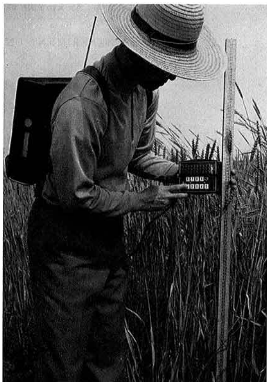
Fig. 2. Measuring with portable device for wireless transmission.
