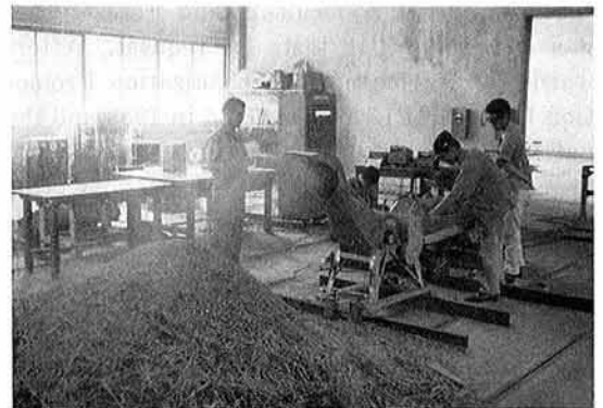
Fig. 2. Cutting performance test of fodder cutter.
