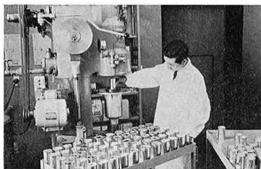
Fig. 7. Packing of seed into moisture-proof containers for extremely long-term seed storage (for seed renewal) in an air-conditioned room of 20–30°C with 30% of relative humidity.
