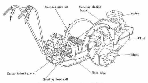
Fig. 4. Transplanting machine with float.
