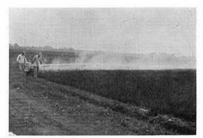
Fig. 2 Travelling type power duster
