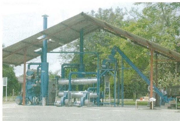
Figure 8. CLAYUCA model for cassava flour processing: artificial drying, continuous process.
