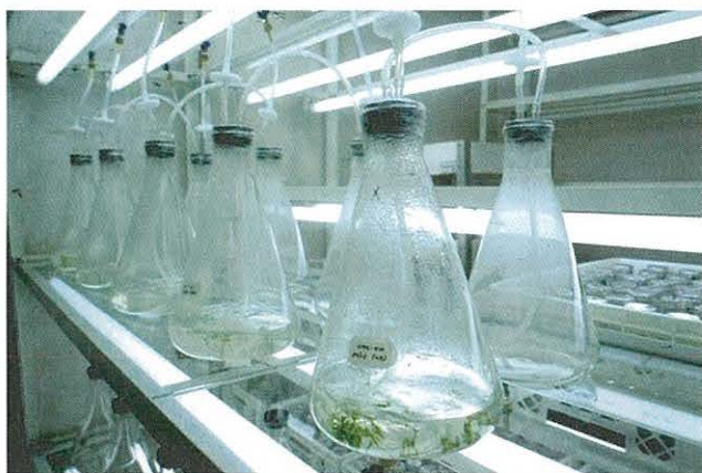
Figure 3. Temporary immersion system for the rapid multiplication of cassava plants.
