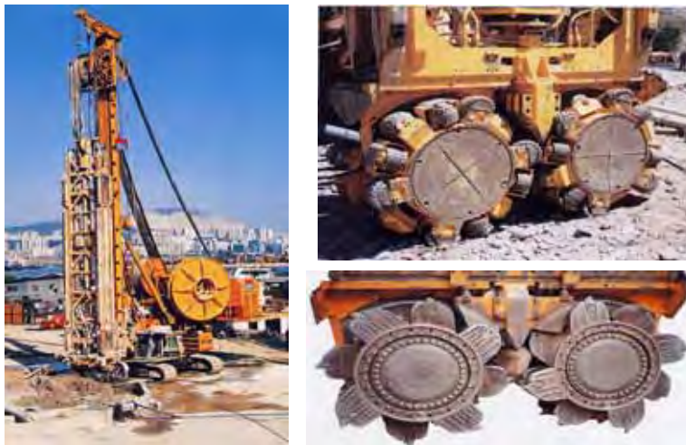
Figure 4.4.70 BAUER Horizontal Two-axial Operating Excavator (Trench Cutter)
