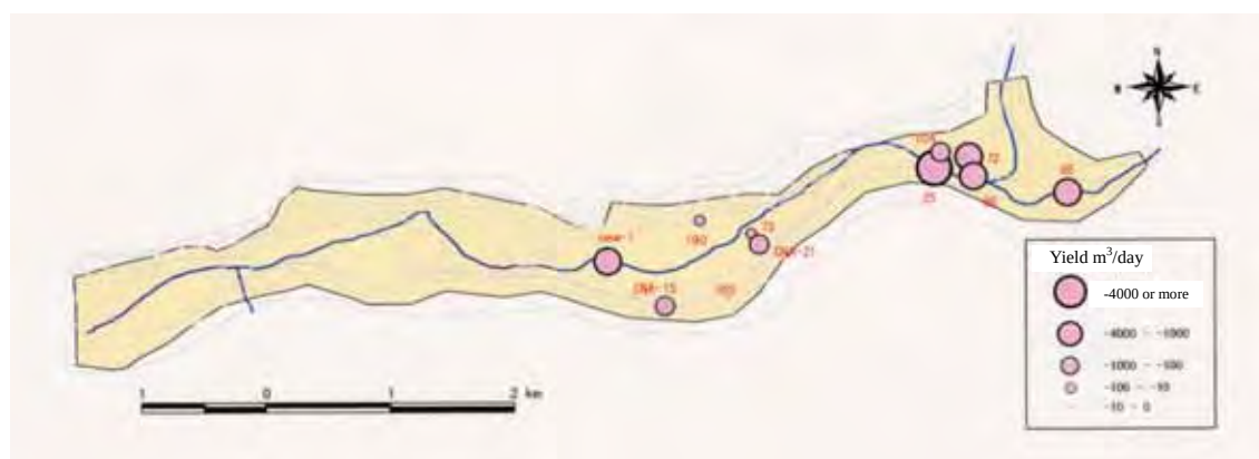
Figure 4.4.61 Pumping Well Locations and Set Water Quantities
