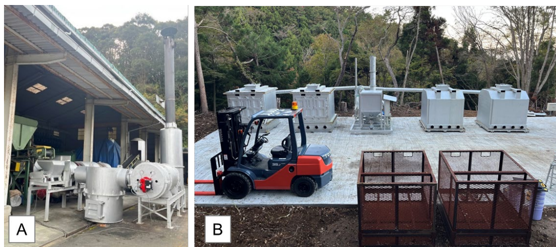
Photo 4.1. Continuous rotary kiln (A), and mobile anoxic pyrolysis units (B). Photo credits: (A) Soil Farm Co. Ltd., and (B) Takatsuki Biochar Energy Lab.
