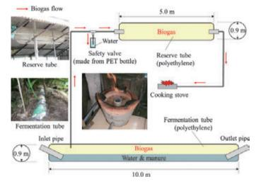
Fig. 1. Plastic biogas digester (BD) system
