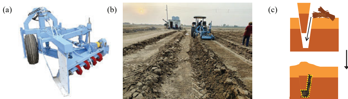
Fig. 1. (a) Cut-soiler, (b) Construction with Cut-soiler, and (c) Schematic diagram
