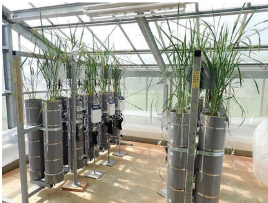
Photo 1. Pipe tests for measuring \text{NO}_3\text{-N} leaching at TARF
