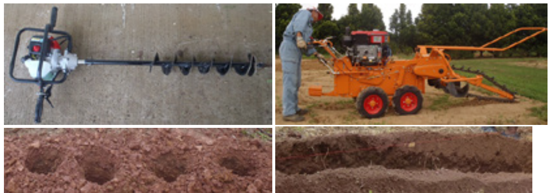
Fig. 1. Gas-powered portable auger (left) and self-propelled trencher (right)
