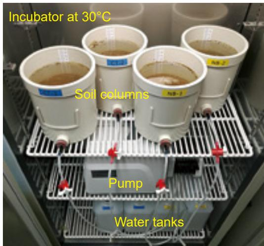
**Fig. 1. Apparatus consisting of soil column systems for the three experiments**
