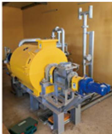
**Fig. 3. External heating U-turn rotary kiln for calcination (Burkina Faso, INERA-Kamboinse)**
