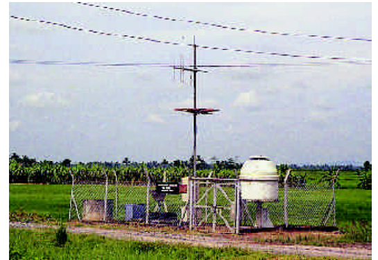
Photo 2. Rainfall station equipped with a VHF radio.
