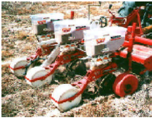
Fig. 2. Seeding with no-tillage seeder
