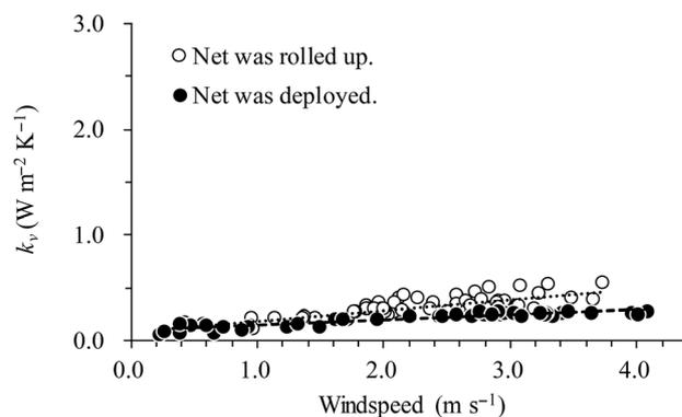
**Fig. 5. Dependency of the leakage heat transfer coefficient on windspeed outside the greenhouse**
