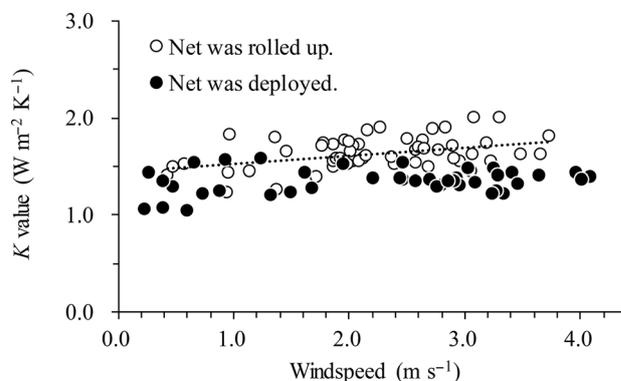
**Fig. 8. Dependency of the overall heat transfer coefficient of the greenhouse cover ( $K$  value) on windspeed outside the greenhouse**
