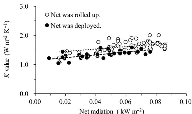
**Fig. 7. Dependency of the overall heat transfer coefficient of the greenhouse cover ( $K$  value) on net radiation outside the greenhouse**
