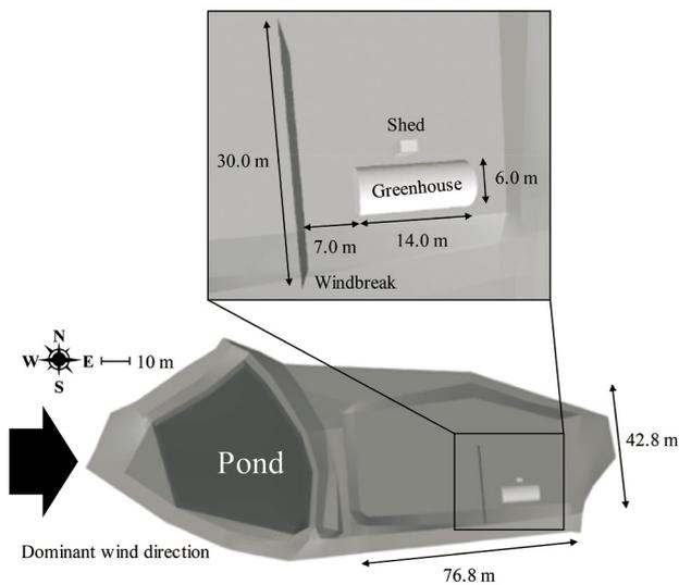
**Fig. 1. Top view schematic of the experimental field**
