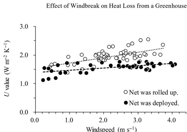
**Fig. 4. Dependency of the overall heat transfer coefficient of the entire greenhouse ( $U$  value) on windspeed outside the greenhouse**
