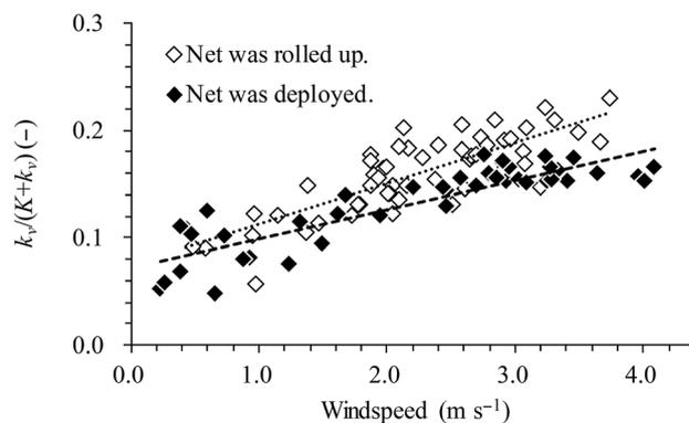
**Fig. 6. Ratio of leakage heat transfer coefficient to the overall heat transfer coefficient ( $U$  value)**
