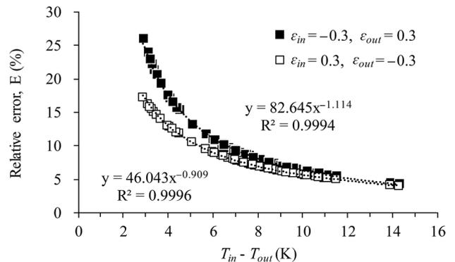
**Fig. A. 1. Influence of the air temperature difference between inside and outside the greenhouse on the relative error of the  $U$  value**
