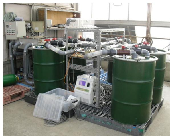
図2 CO<sub>2</sub>回収・施用装置
