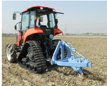
Fig. 2. Drilling unit in operation
