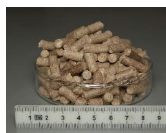
Fig. 5. Pellets produced from dry matter of JES1
