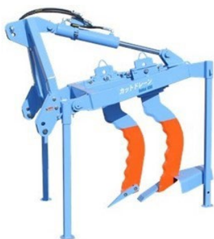
Fig. 1. Drilling unit of “Cut Drain”
