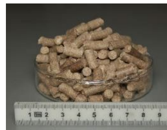
Fig. 5. Pellets produced from dry matter of JES1
