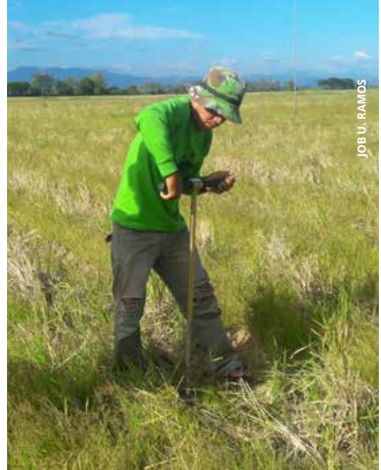
Sampling for soil analysis and soil data using “auger”, a 1-m device that can get five samples in every 20cm depth.
