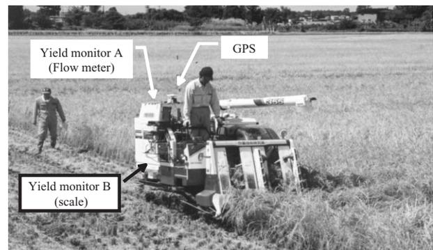
**Fig. 8. Yield monitoring combine with GPS and dual yield monitoring system**
