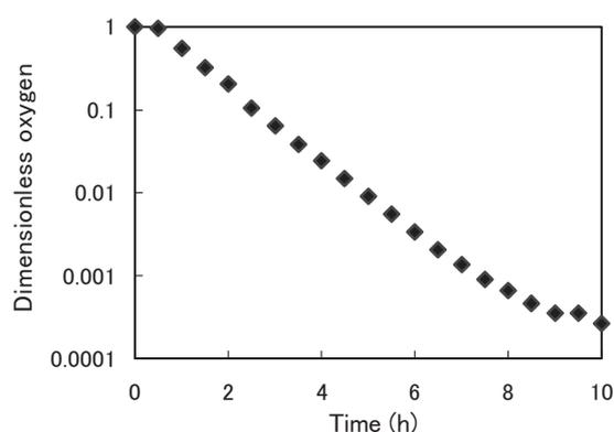
Fig. 2. The characteristic of gas exchange of the chamber
