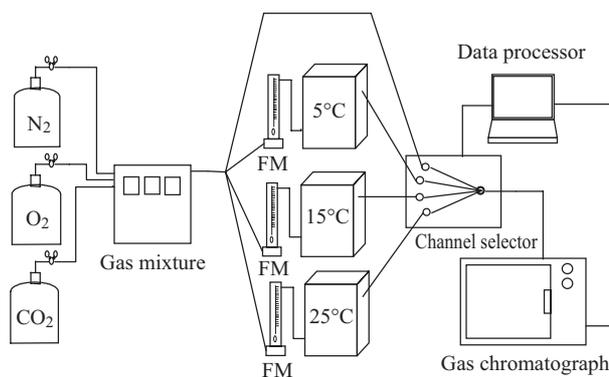
**Fig. 1. The schematic of flow through system**
