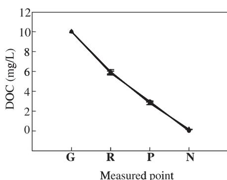
**Fig. 3.** Dissolved ozone concentration (DOC) of OW at the outlet of the ozonated-water generator (G), in the reservoir (R), at the pipe end (P), and at the nozzle outlet (N) when released with the 5 and 50  $\mu\text{m}$  nozzles
