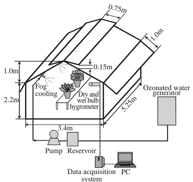
Fig. 1. Schematic diagram of the experimental setup used for ozonated water-fog cooling
