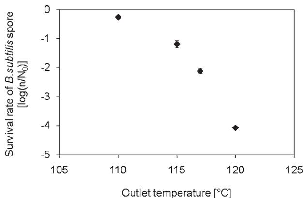
**Fig. 3. Viability loss of *B. subtilis* spores in orange juice using HEF-AC at different outlet temperatures**
