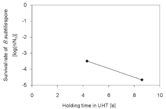
**Fig. 4. Viability loss of *B. subtilis* spores in orange juice using UHT at different flow rates**
