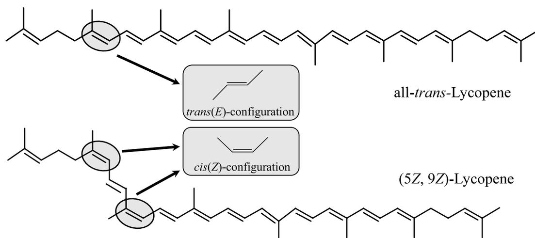
Fig. 3. Structure of geometrical isomers of lycopene
