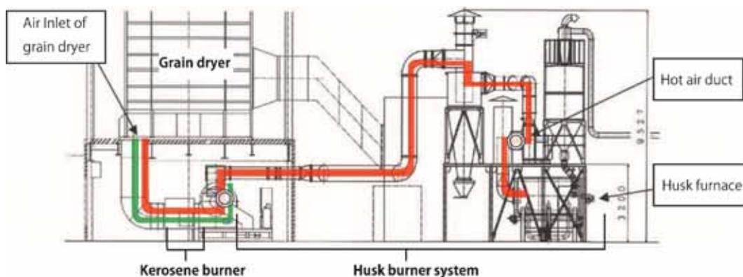
Fig. 3. Layout of the husk burner system, kerosene burner and grain dryer
