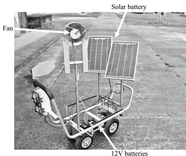
Fig. 10. Solar-powered forced airflow system
