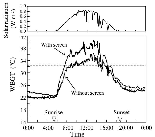
**Fig. 8. WBGT values in a greenhouse covered with a 0.6 mm mesh screen**
