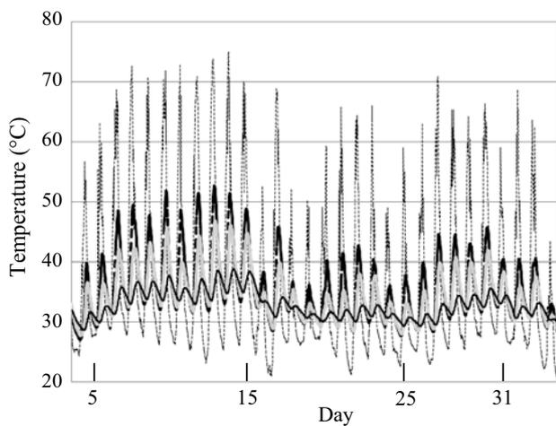
**Fig. 7. Temperature of solarized soil at different depths during August 2004**
