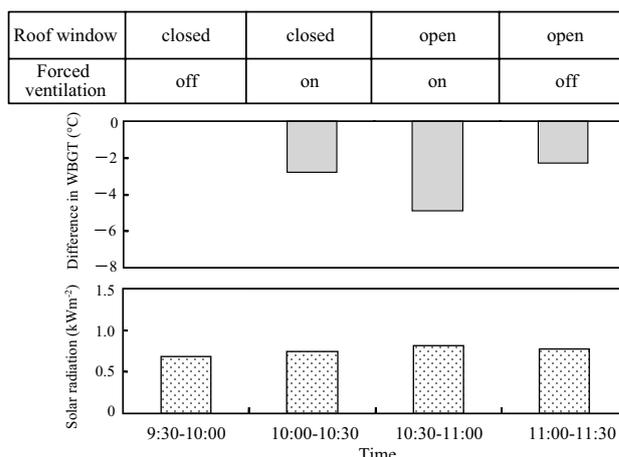
Fig. 11. Effects on WBGT of forced ventilation and roof windows installed in a greenhouse
