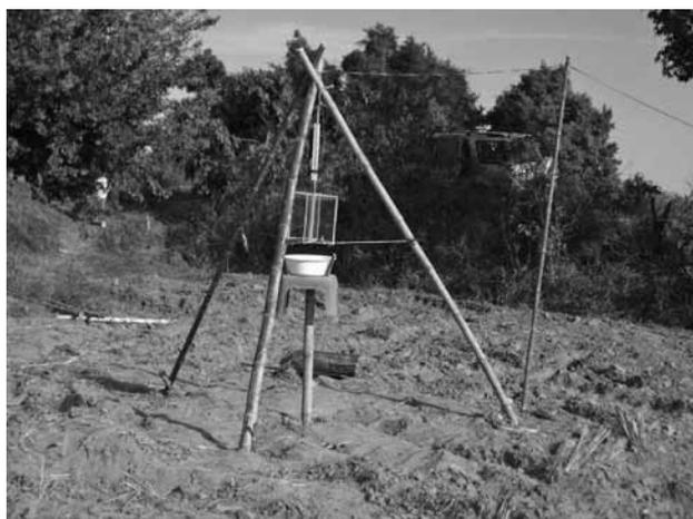
**Photo 1. A light trap in the experimental field**
