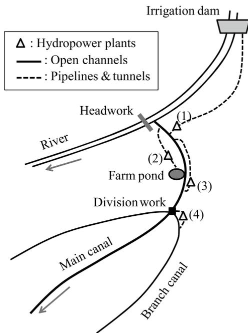
**Fig. 1. Schematic diagram of possible hydropower generation sites in an irrigation canal system**
