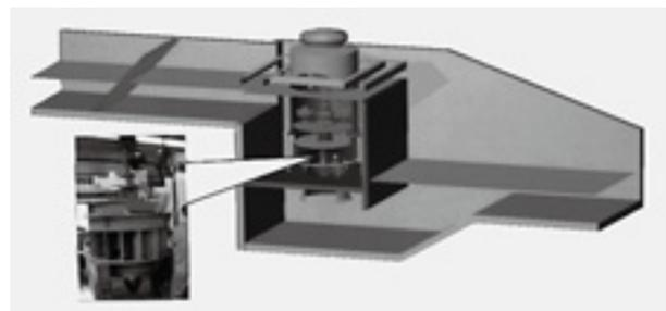
**Fig. 7. Water turbine (Kaplan) installed at a drop along an open channel (Tochigi Pref.)**
