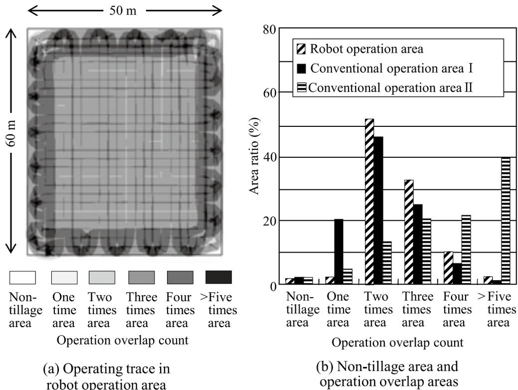
**Fig. 6. Operating trace of the robot soil paddling and the ratio of the overlap area**
