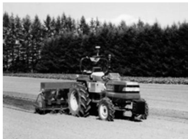
Fig. 3. Field test of the robot wheat seeding
