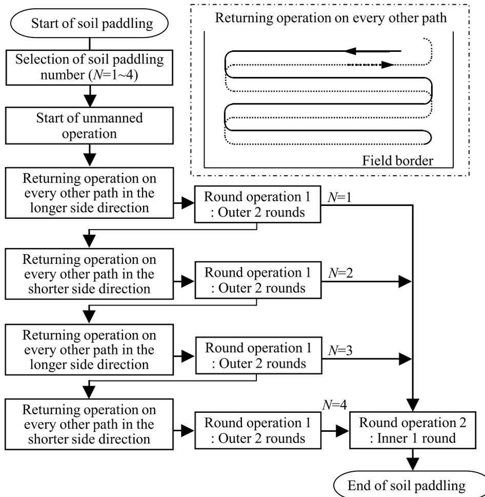
Fig. 4. Returning operation method of the robot soil paddling and the flow of operation software for soil paddling
