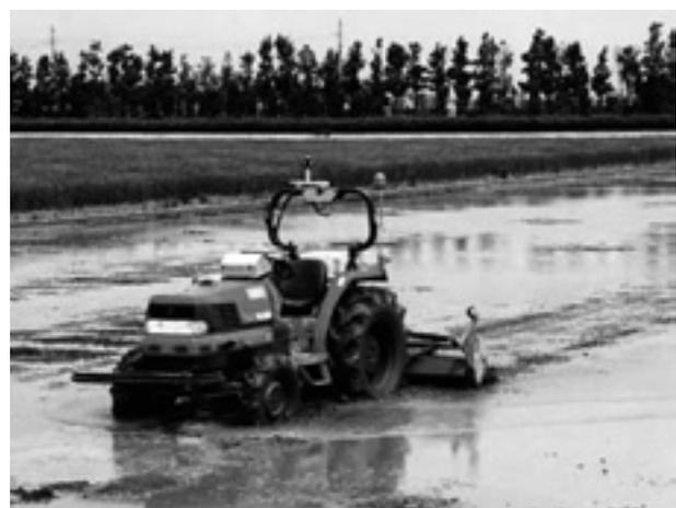
Fig. 5. Field test of the robot soil paddling
