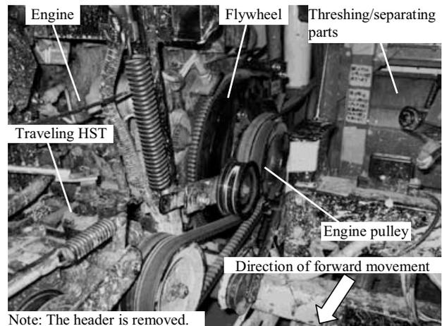
Fig. 1. View of the power transmission part of a head-feeding combine
