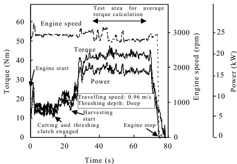
**Fig. 5. Fluctuation of torque during harvesting operation**
