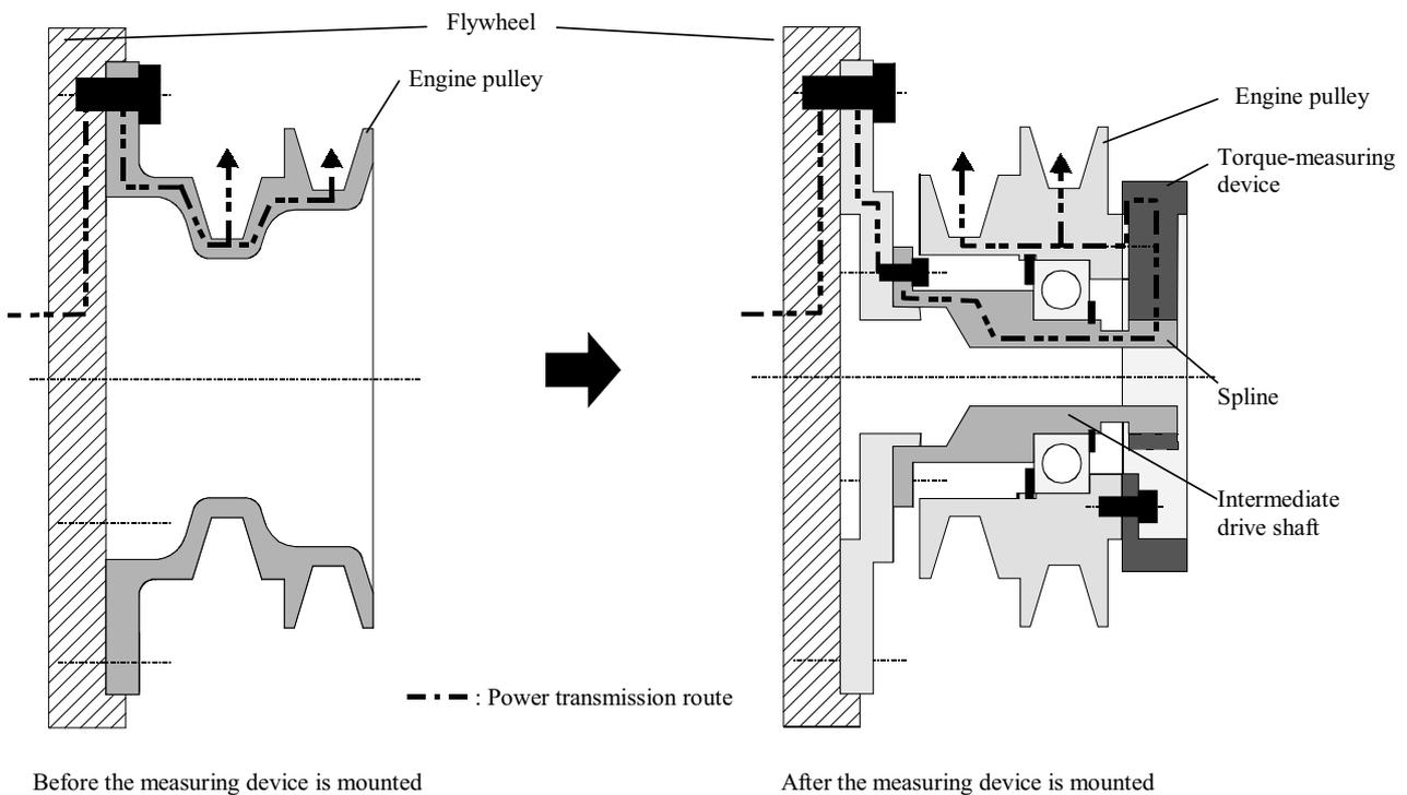
Fig. 2. Overview of torque-measuring device structure
