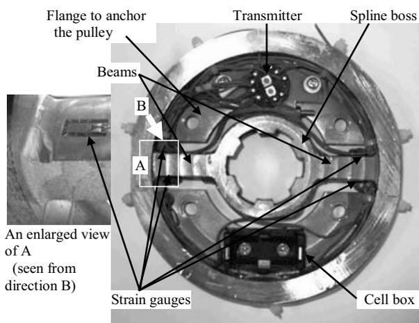
Fig. 3. Overview of the measuring part (seen from the right in Fig. 2)
