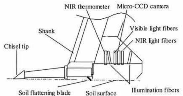
Fig. 7. Soil penetrator and optical fiber probes
