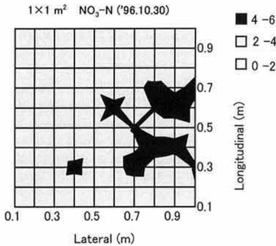
Fig. 4. Map of nitrate nitrogen content at 5–15 cm depth within a 1×1 m<sup>2</sup> area (0.1 m grid spacing)
