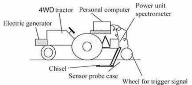
Fig. 6. Portable spectrophotometer system developed for *in situ* soil sensing
