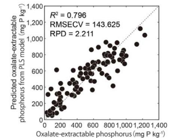
Fig. 2. Relationship between observed and predicted values of soil oxalate-extractable P using the PLS model
