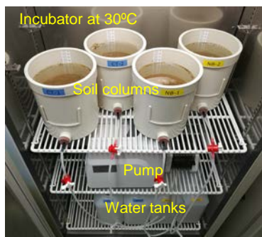
図1 土壌カラム実験装置 Fig. 1. Apparatus consisting of soil column systems for the three experiments Water is leached at a fixed rate (1.73 cm day -1 ) by the pump.
