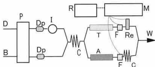
Fig. 3. Flow injection analysis system for ester-type catechins
