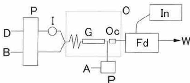
Fig. 5. Flow injection system for GABA analysis
