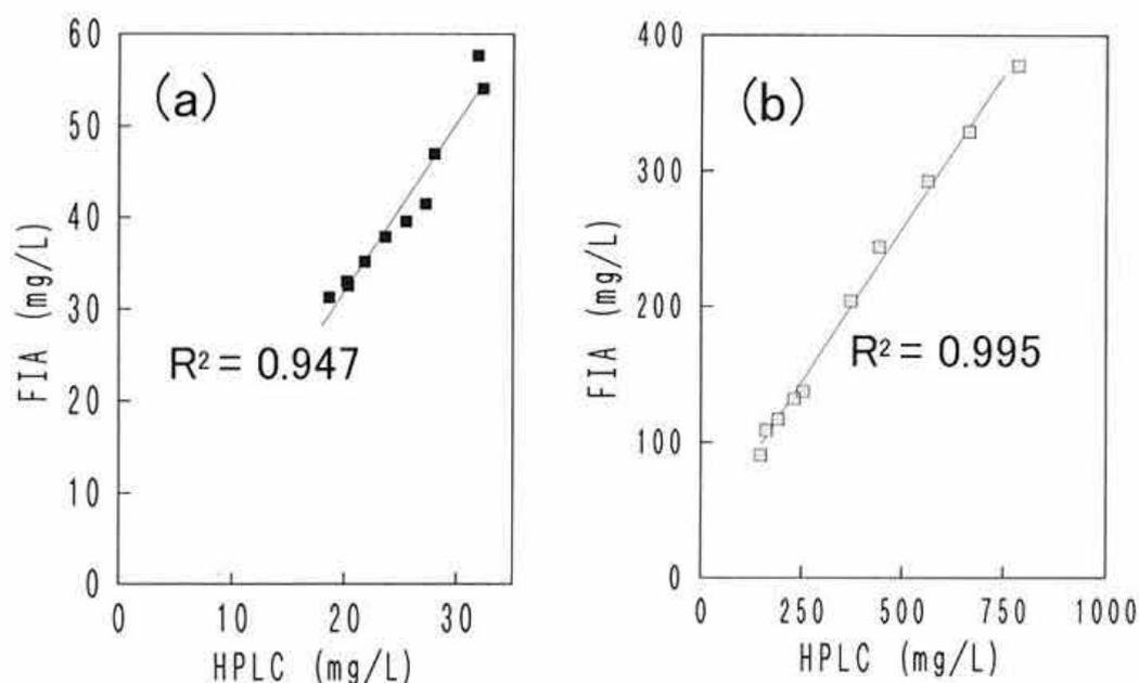
**Fig. 2. Comparison of the composition of tea infusions determined by FIA and HPLC methods**
