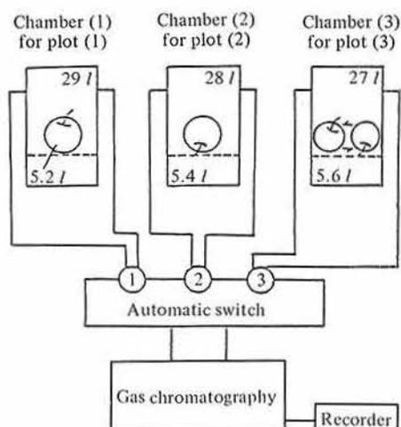
Fig. 4. Ethylene monitoring system
