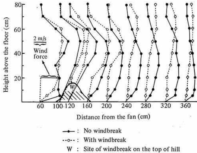
Fig. 7. Vertical profile of wind force as influenced by windbreak (model experiment)
