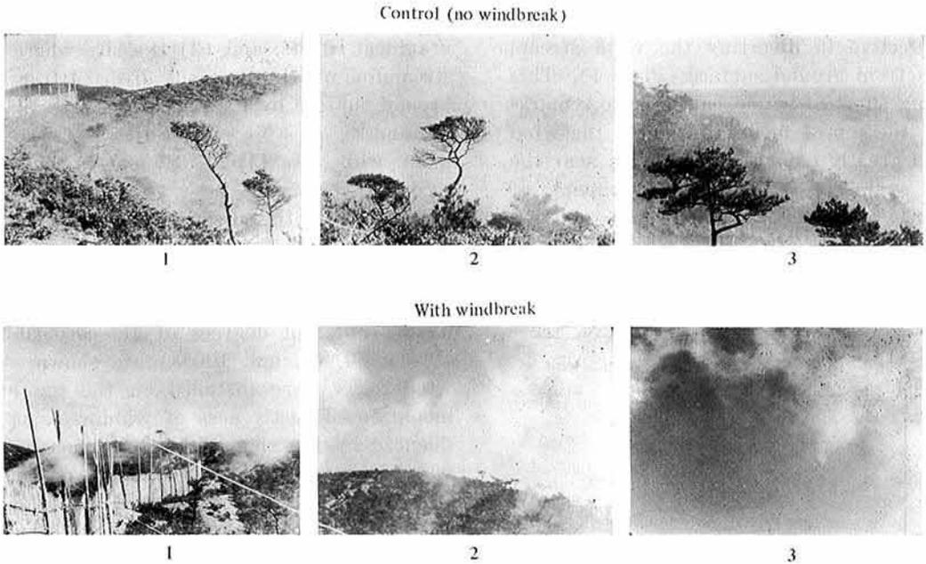
Plate 1. Wind diverted upward by a windbreak installed on the top of a mountain. Wind movement is shown by the movement of smoke and can be traced by following the pictures from 1 to 3.
