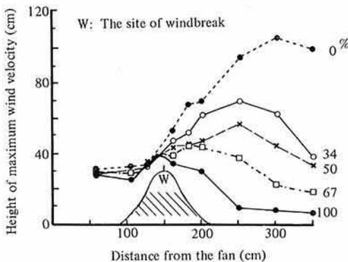
Fig. 8. Relation of air-permeability of windbreak to the effectiveness of windbreak (model experiment)
