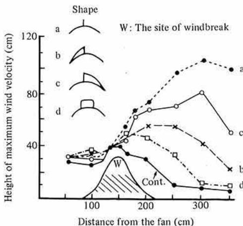
Fig. 9. Relation of shape (cross section) of windbreak to the effectiveness of the windbreak (model experiment)
