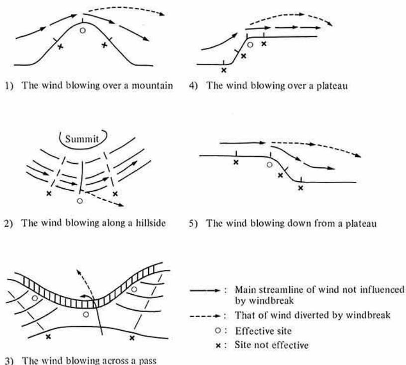
Fig. 6. Effective sites for installing windbreaks
