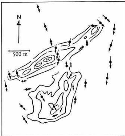
Fig. 2. Direction and force of wind blowing around a hill in flat land
