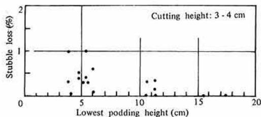
Fig. 3. Relation between the lowest podding height and stubble loss—Model BH795
