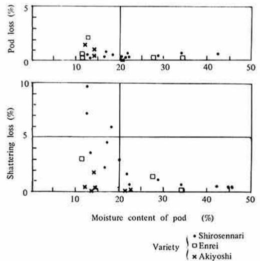
Fig. 2. Relation between moisture contents of pods and shattering loss, or pod loss — Model BH795
