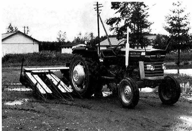
Plate 3. Two-row soybean reaper (4-wheel tractor-mounted type)—Model M2-KB
