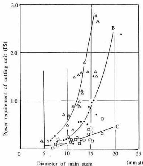
Fig. 4. Comparison of power requirement of various cutting units
