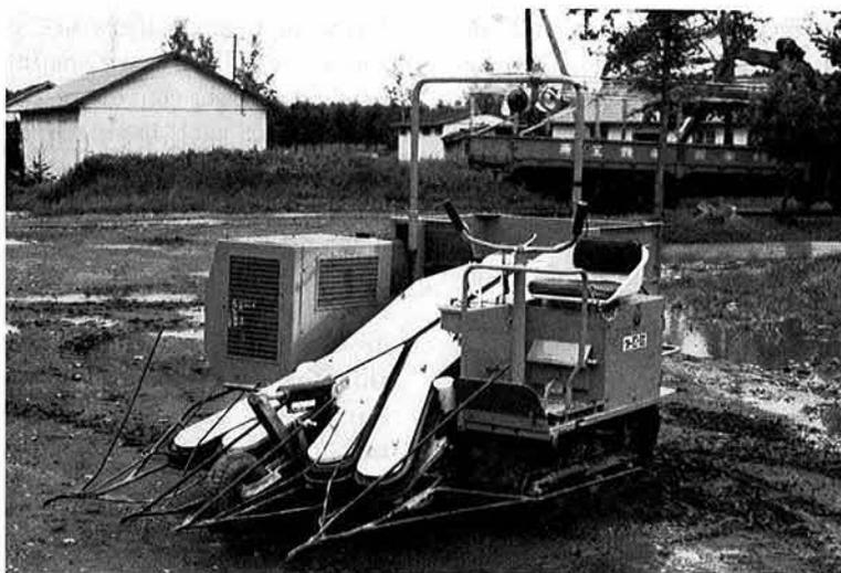
Plate 2. Two-row soybean reaper (self-propelled type)
