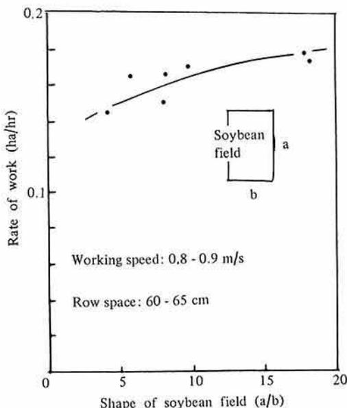
Fig. 5. Relation between shape of soybean field and rate of work of 1-row soybean reaper—Model BH795
