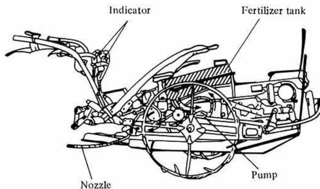
Fig. 1. Rice seedling transplanter equipped with an applicator for simultaneous application of paste-like fertilizer
