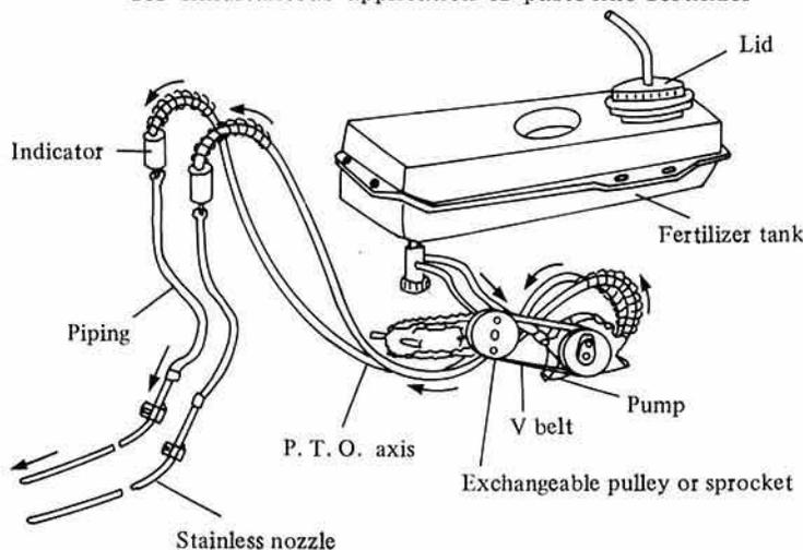
Fig. 2. Applicator for paste-like fertilizer
