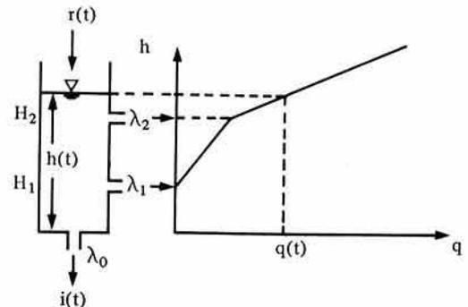
$$\begin{aligned} q(t) &= q_1(t) + q_2(t) & h(t) &: \text{Storage (mm)} \\ q_1(t) &= (h(t) - H_1) \cdot \lambda_1 & \lambda_0 &: \text{Coeff. of seepage hole} \\ q_2(t) &= (h(t) - H_2) \cdot \lambda_2 & \lambda_1, \lambda_2 &: \text{Coeff. of discharge hole} \\ i(t) &= h(t) \cdot \lambda_0 & r(t) &: \text{Input (mm)} \\ r(t) - q(t) - i(t) &= \frac{dh}{dt} & i(t) &: \text{Output seepage (mm)} \\ & & q(t) &: \text{Output discharge (mm)} \end{aligned}$$
