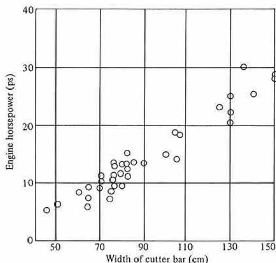
Fig. 1. Relationship between width of cutter bar and engine horsepower
