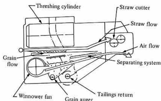
Fig. 2. Cross-section of the threshing device of combine harvester
