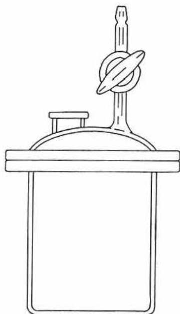
Fig. 1. A vessel used for acetylene reduction assay
