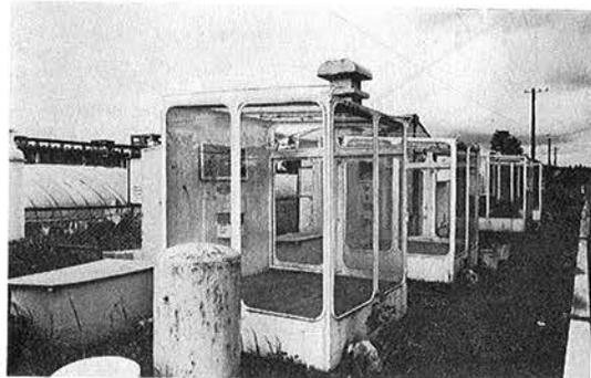
Plate 2. Experimental facility to measure plant growth and dry matter production under natural light with chronic exposure to  $\text{SO}_2$  gas.
