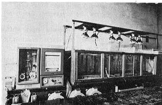
Plate 1. Experimental facility to measure photosynthesis under artificial light with  $\text{SO}_2$  gas treatment
