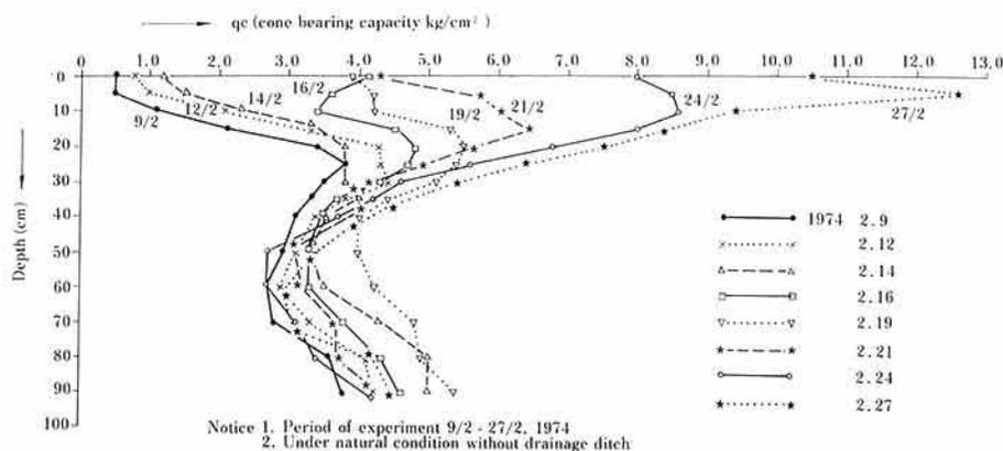
Fig. 1. Changes of qc in a course of soil drying.
