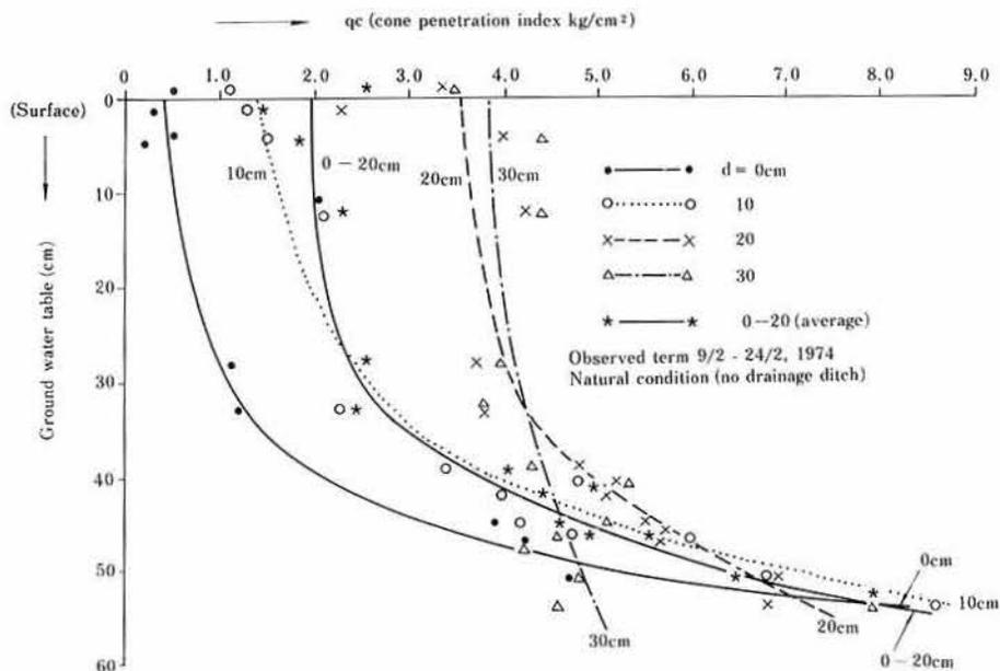
Fig. 2. Relationship between ground water table and cone penetration index at different depth
